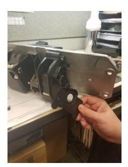
Step 2: Remove plate where Mcor is mounted
